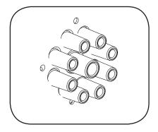
The liquid soap connection consists of **8** connections for liquid soap.
