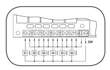
On machines equipped with a liquid soap connection, connect the wires *directly on the print board* next to the ground wire connection (option). Connect as indicated on the wiring diagram.
