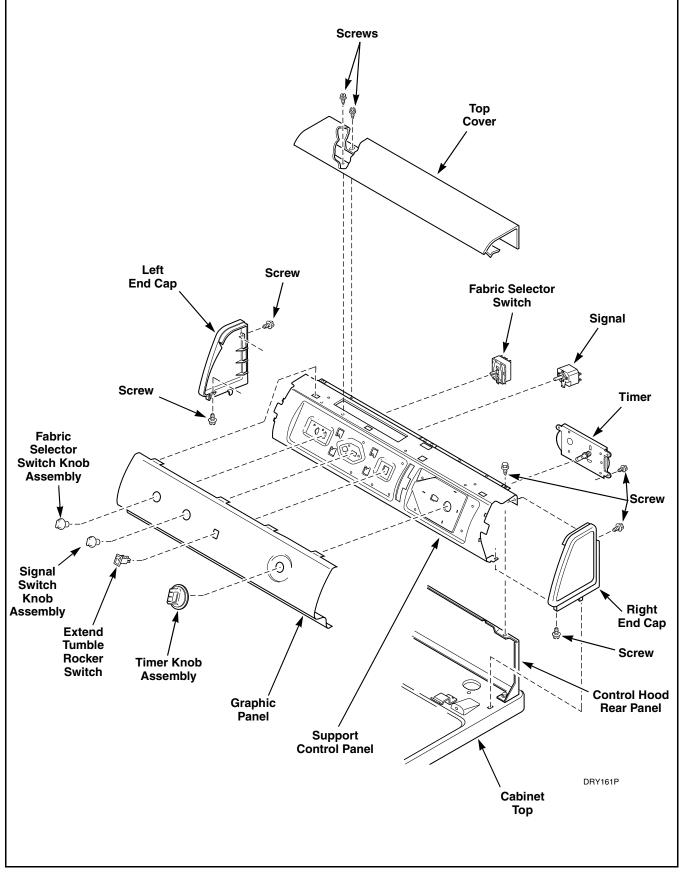
Figure 5 GRAPHIC PANEL, CONTROL HOOD AND CONTROLS – REAR CONTROL DRYERS
