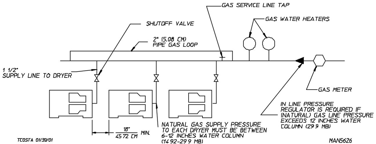
Consistent gas pressure is essential at **ALL** gas connections. It is recommended that a 2-inch (5.08 cm) pipe gas loop be installed in the supply line servicing a bank of dryers. An in-line pressure regulator **must be** installed in the gas supply line (header) if the (natural) gas pressure exceeds 12.0 inches (29.9 mb) of water column (W.C.) pressure.
