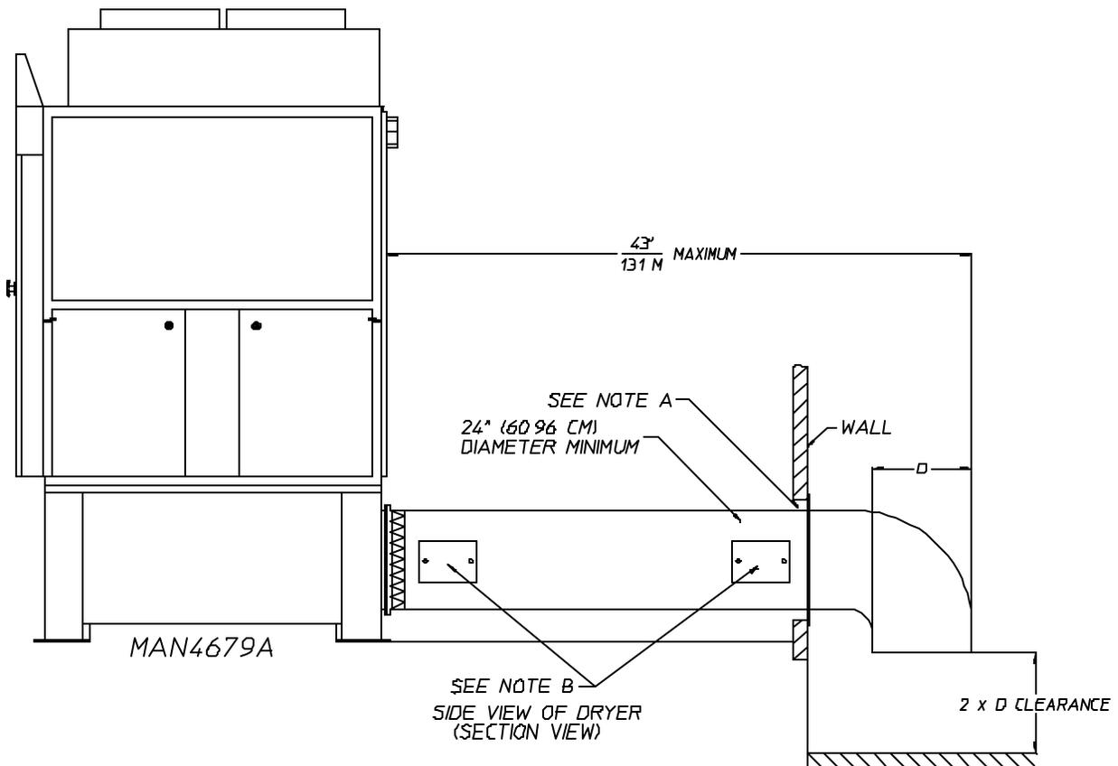
NOTE "A"- OPENING MUST BE 2-INCHES (5.08 CM) LARGER THAN THE DUCT (ALL THE WAY AROUND) THE DUCT MUST BE CENTERED WITHIN THIS OPENING
