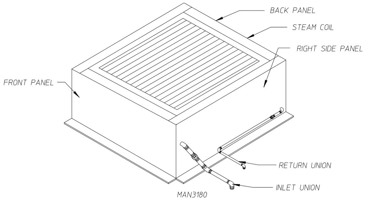
VIEW OF STEAM COIL w/ DAMPER REMOVED
