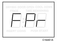
When "FPr" appears in the VFD, press the START pad. The current number of coins required to fulfill the NO HEAT vend price will appear in the VFD.
