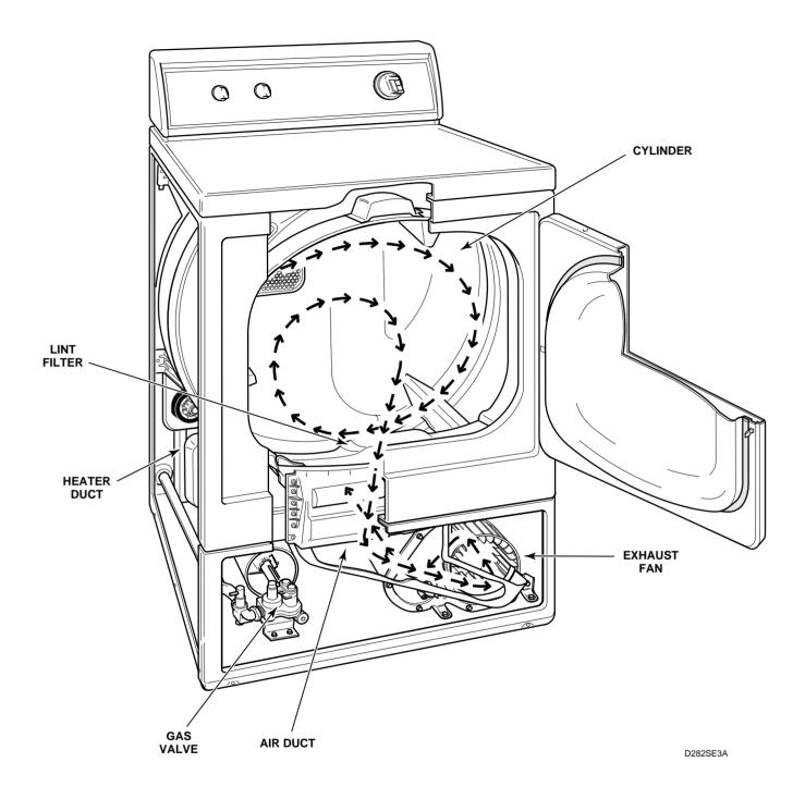
The dryer uses heated air to dry loads of laundry. When the motor is started, the exhaust fan pulls room temperature air in through louvers at the rear of the dryer and over the heat source (burner flame for gas and heating element for electric). The heated air moves through the heater duct and into the cylinder, where it circulates through the wet load. The air then passes through the lint filter, air duct, and exhaust fan, where it is vented to the outdoors.
