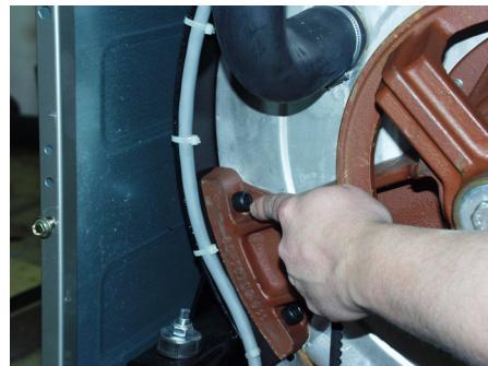
10. If necessary, tighten the shock absorbers' mounting bolts.
