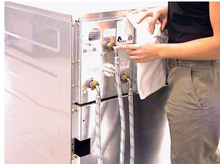
2. Inspect the steam hose connections for leaks (where applicable).
