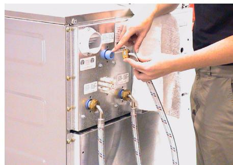
4. Remove the top panel and check the supply dispenser hoses for leaks.
