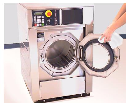
5. Shut off the main water, steam and power connections at the end of each day. Do not change the setting of the water inlet taps on boiler-fed machines once these have been installed.
