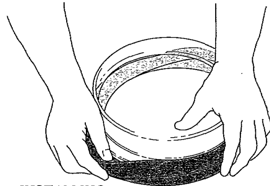
INSTALLING GASKET ON GLASS
