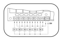
The two connectors on the right give a tension of  $220V \sim (max. 4A)$  which can be applied to drive  $220V \sim soap$  pumps. If more than 4A is required, *an external tension* will have to be used.
