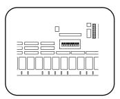
In this test it is possible to verify whether the switches are open or closed. In case of a machine type HF, WE245/304, or WE "high spin", these DIP switches are used to determine how long the spin motor is activated during acceleration to the distribution speed.
