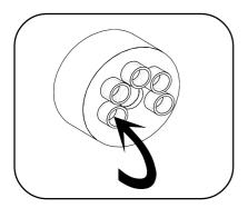
A rubber connection has been placed over the air break opening at the back of the machine. There are *5 holes* in this rubber connection, through each of which a liquid soap hose can be driven *(S1...S5)*. Press the hoses until they appear well *inside the soap dispenser*.
