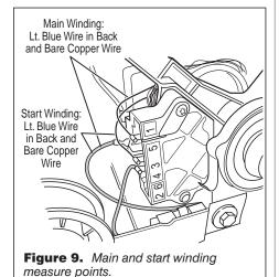
**6.** Using figure 9, check for the resistance values of the motor's Main and Start winding coils as shown in the following table.
