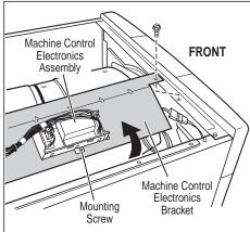
**Figure 16.** Remove machine control electronics from mounting bracket.
