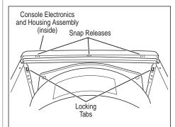
**Figure 18.** Remove the console panel to access the console electronics and housing assembly.
