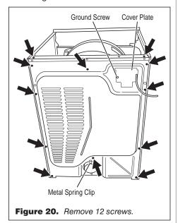
**5.** Remove the ten screws on the rear, and two screws on the top of the back panel. Pull the back panel off the machine. See figure 20.
