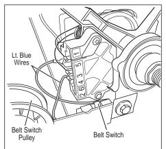
Figure 10. Checking the belt switch.
