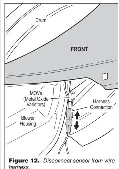
5. Access the machine control electronics. See Accessing & Removing the Electronic Assemblies, page 10. Remove connector P13 from the circuit board. Check the main harness connections between the sensor harness and machine control for a short or open circuit.
