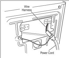
**Figure 5.** Power cord-to-wire harness connection for gas dryer.
